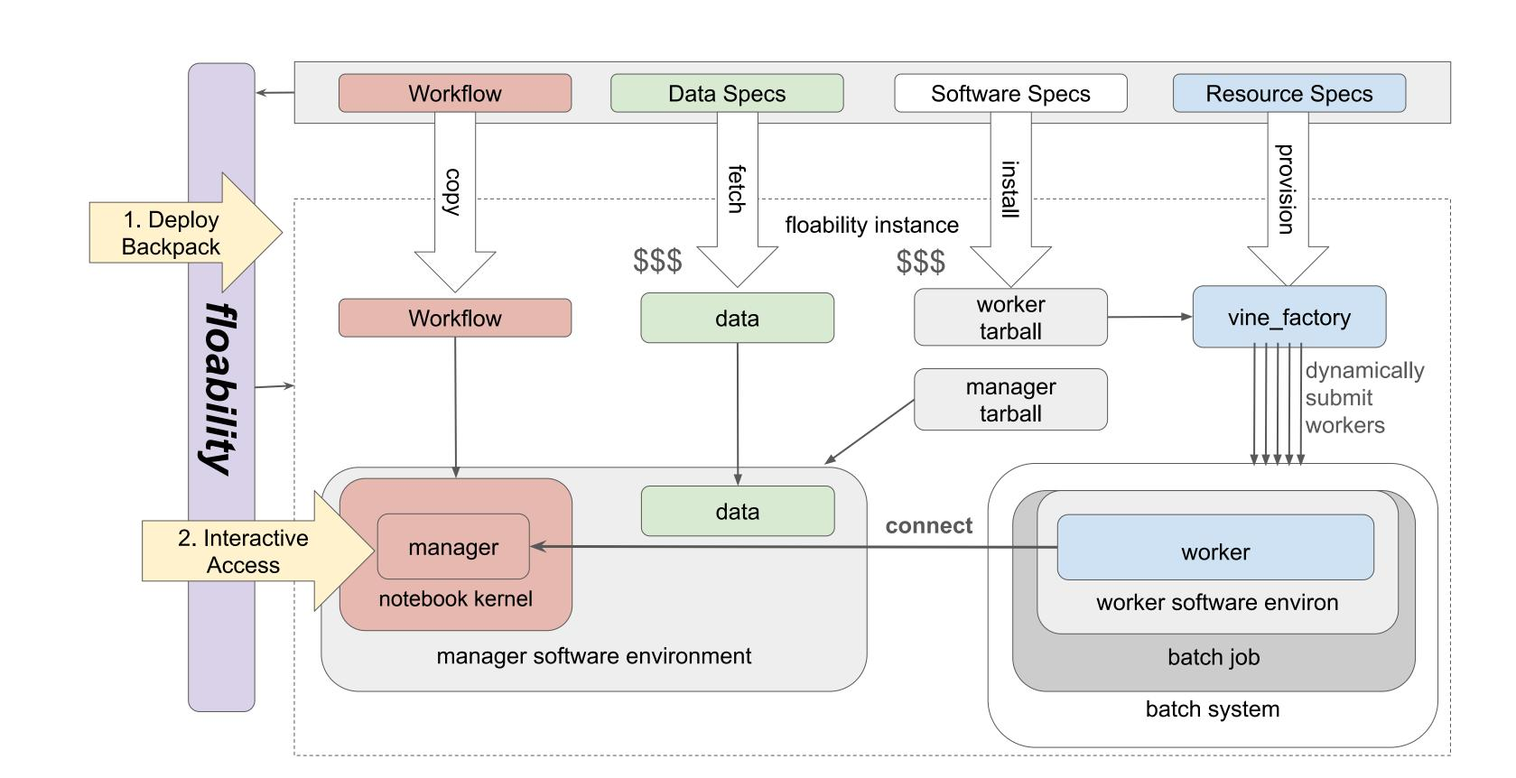
Floability architecture consists of a manager running on the head node and multiple worker processes running on compute nodes. A factory process is responsible for launching and dynamically scaling workers in the cluster.
