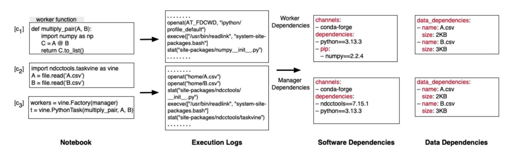
Floability *audit* uses system call tracing to extract manager and worker software packages, which are then validated to produce an environment file with precise versions.
